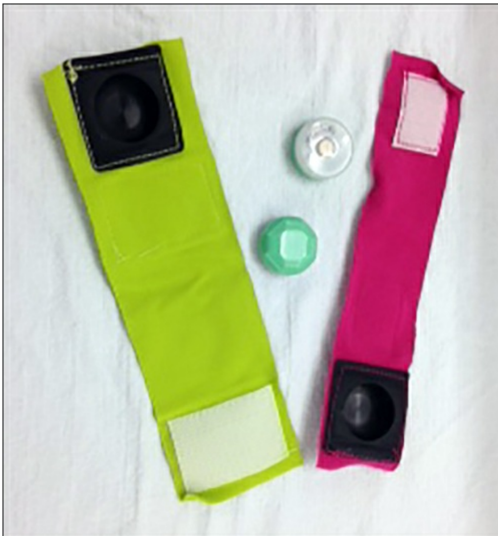
A Tamper Sensing tag is applied to a newborn's lower leg using a stretchable leg band with a Velcro strip shortly after birth.
